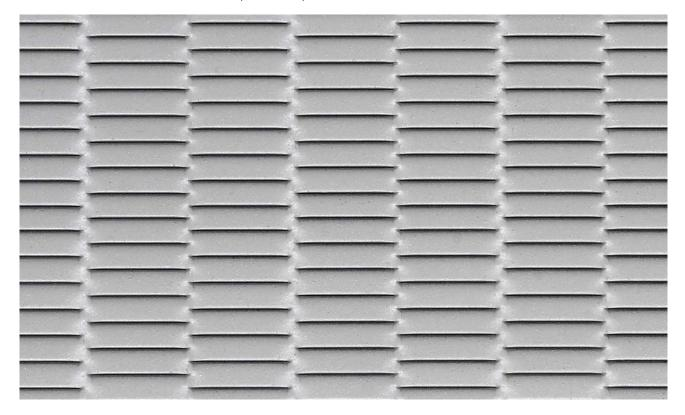
LW Pitch:63.00mmStrand Width:4.00mmSW Pitch:8.50mmThickness:0.90mmWeight:6.64 kg / m2Open Area:6%
